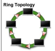
Each networked computer is connected to two others in a closed ring. Sometimes two rings are used to increase the *fault tolerance*
